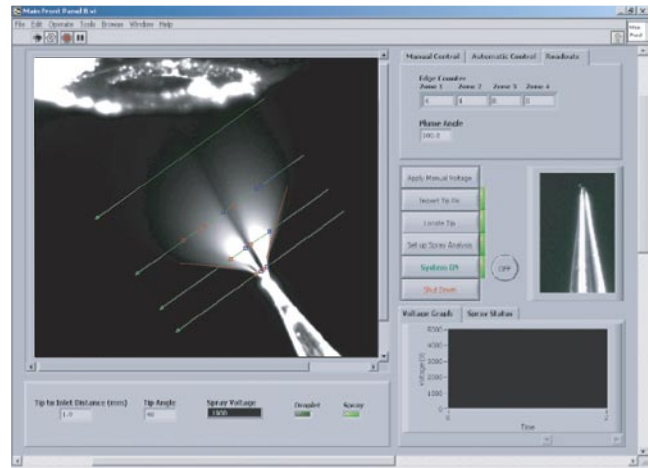
Figure 8 - Spray analysis of the multi-jet mode by the automated control system software
