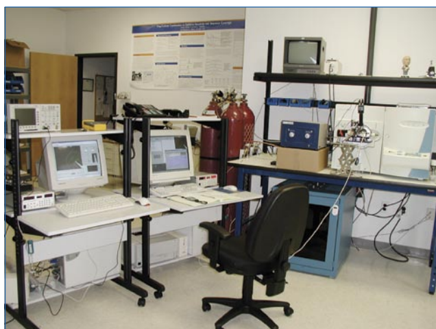
Figure 1 – LCQ Deca™ (Thermo Electron) equipped with an automated ESI control system. The system is controlled independent of the mass spectrometer by a PC (left). The mass spectrometer and the NanoLC (Eksigent Technologies) are controlled by a second computer (center).
