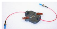
A microfabricated 90 nL (5 mm pathlength) flow cell employing fiber optic coupling provides sensitive detection for quantitative UV absorbance measurements in micro-LC. The cell, which is easily exchanged on the instrument, provides very low peak broadening. When combined with the newly designed CCD-based detector, the system provides low UV noise, and linear response to greater than 2AU. A 10mm pathlength cell (180 nL) has also been used.
