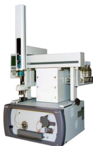
Photograph of the ExpressLC-Ultra system for ultra high pressure micro-LC. The system provides automated solvent selection for a 10,000 psi binary gradient delivery system, a unique small volume sample injection system, an industry standard autosampler with high sample capacity, a high performance column oven, and a new, sensitive CCD based UV detection system.
